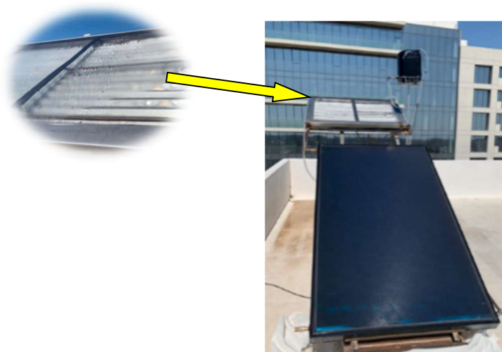
Fig 3. Final pilot scale unit with hybrid desalination module with water condensation on glass cover.
