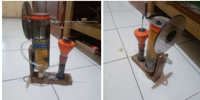
Figure 2. Completed gamma-type Stirling engine prototype constructed from recycled materials: (a) front view showing flywheel and connecting rod, (b) top view showing displacer chamber and power piston orientation, (c) side view showing heat source placement below the hot chamber.
