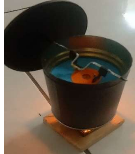
Figure 1. Small-Scale Gamma-Type Stirling Engine
